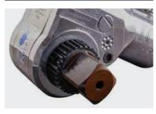
The ICE can automatically release itself when locked on a bolt. This reduces unplanned interruptions in the bolting process.
